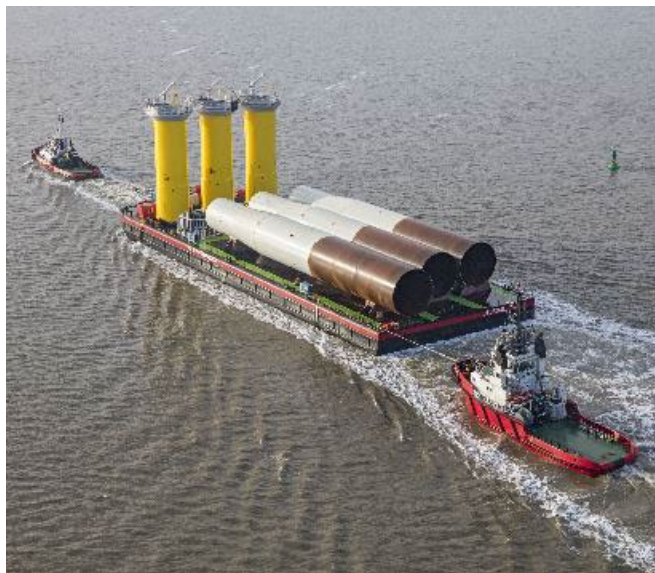
Figure 3-1. Tug and Barge Feeder System for Foundation Transportation Source: Wagenborg.com
